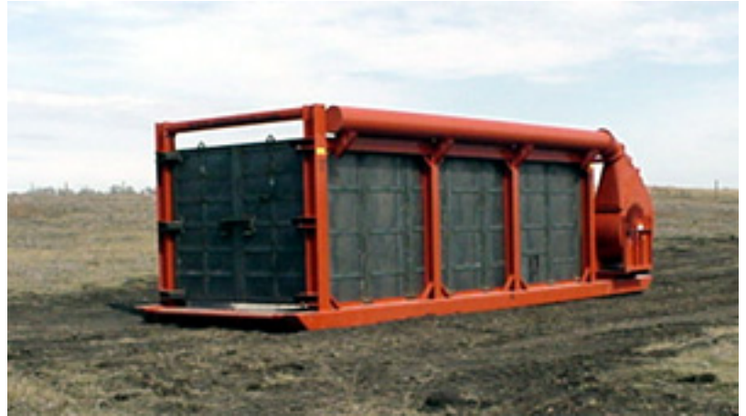
Air curtain incinerator
